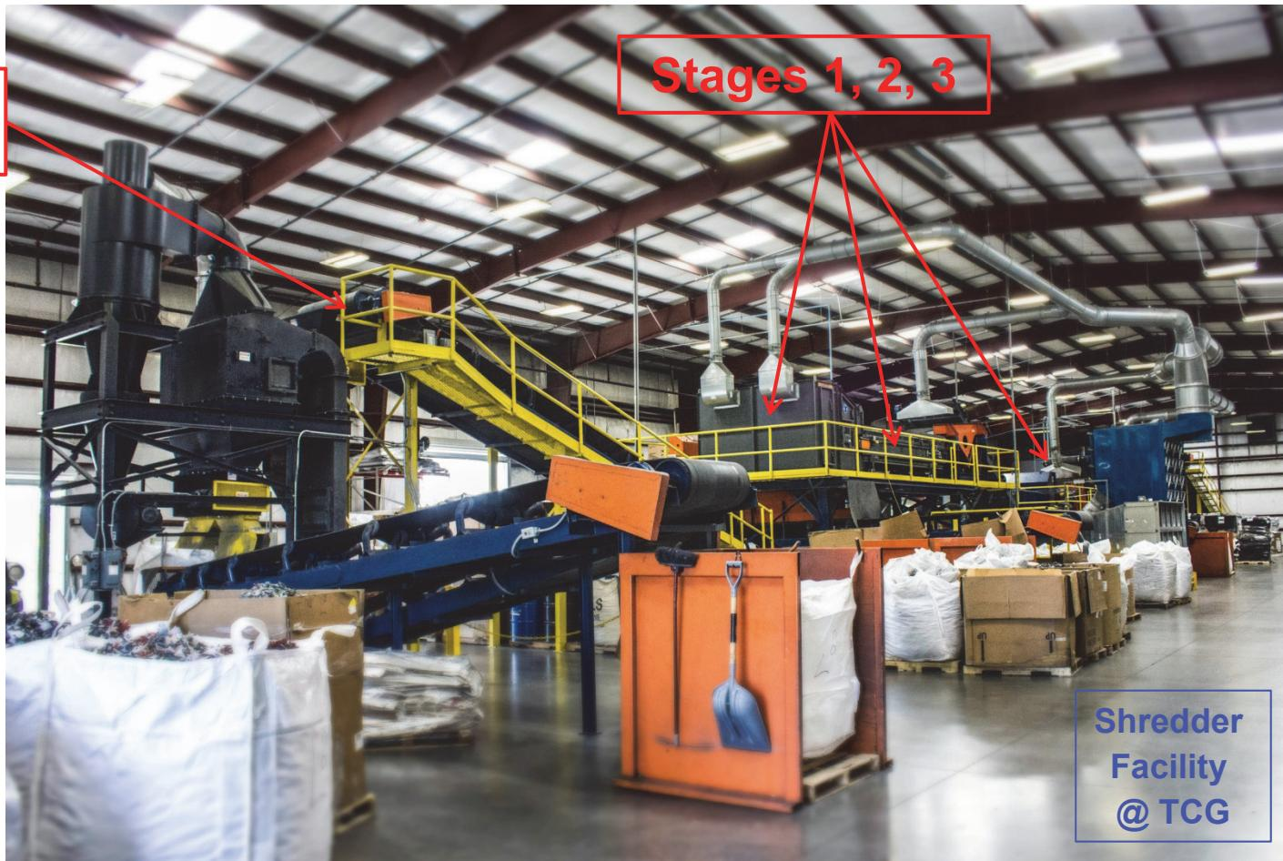
Automated Industrial shredder- *Sorts & bins de-constructed materials*
