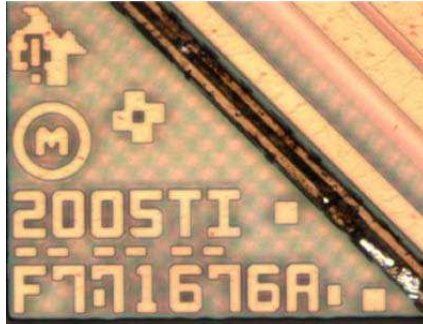
Fig. 8. Die marking on a Texas Instruments (TI) 65 nm processor [Quirk 2013].
